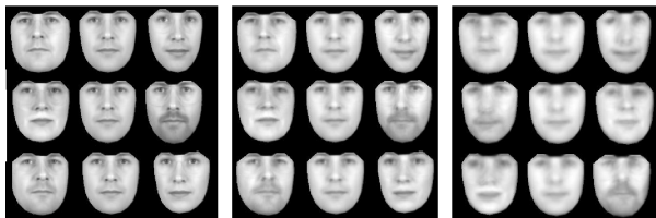
Figure 4. Model constructed from ground-truth annotation: left, and models constructed with increasingly degraded registration: centre and right (variation of \pm 2.5\sigma_0 ) in first three modes
